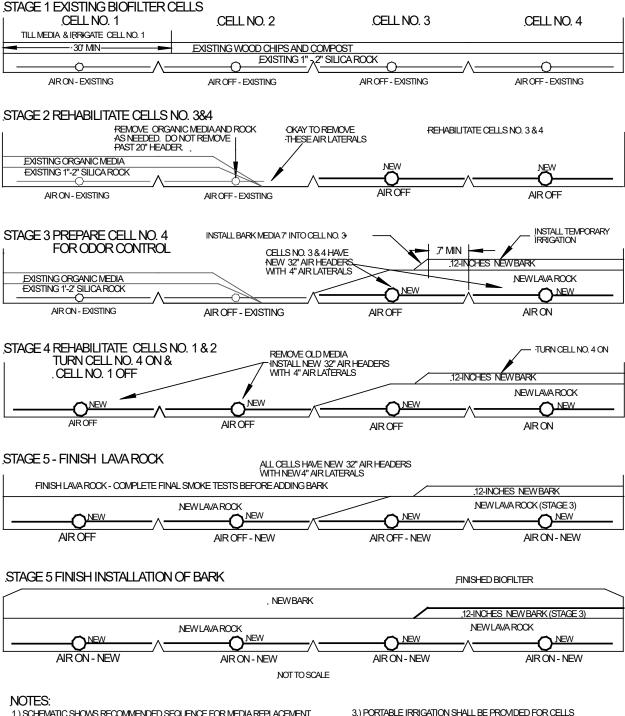
1.) SCHEMATIC SHOWS RECOMMENDED SEQUENCE FOR MEDIA REPLACEMENT . ONLY. THIS STAGING WILL PROVIDE ODOR CONTROL DURING THE CONSTRUCTION
